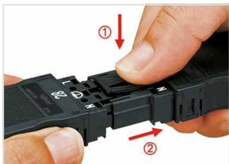
Locking lever, manually operated: • Push on locking lever • Pull the connectors apart
