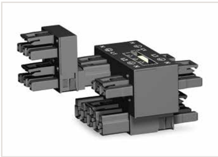
An additional h-distribution connector doubles L1. This results in the following connection options: L1/L1/L2/L2/L3 with jumper in position L2 L1/L1/L2/L3/L3 with jumper in position L3
