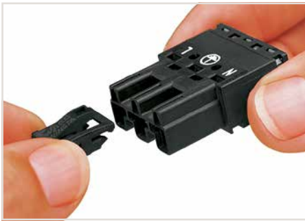
Snap on locking lever – observe direction (picture shows 3-pole plug).
