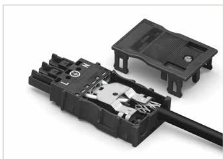
First insert the wired connector into strain relief housing, then snap cover and tighten screw.
