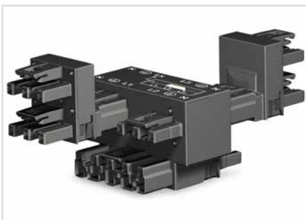
Additional h-distribution connectors double L1 and L3. This results in the following connection option: L1/L1/L2/L2/L3/L3 with jumper in position L2 Notice: h-distribution connectors can only be plugged on L1 and L3.
